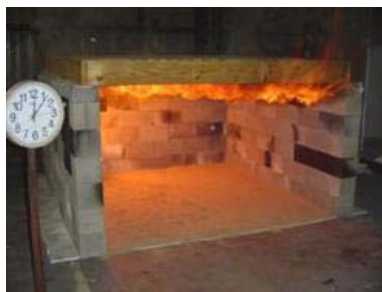
6:00 Minutes: Steady Flames Exiting The Front Of Crawl Space
