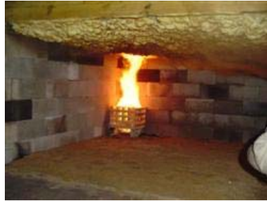
1:40 Minutes: Flames impinging foam surface no ignition of foam.
